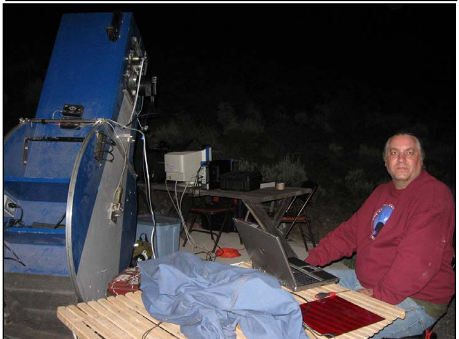
Dan Gray and his 14 inch alt-az robotic telescope, affectionately called "Lollipop" (for obvious reasons). Dan was working to fully automate near infrared aperture photometry.
