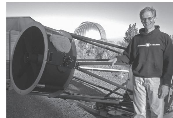
Figure 4: Howard Banich and his portable 28-inch computer controlled telescope. He can unload it and set it up, by himself, in about ten minutes.
