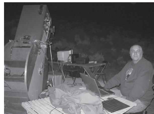
Figure 8: Dan Gray and his 14-inch alt-az robotic telescope, affectionately called "Lollipop" (for obvious reasons). Dan was working to fully automate near infrared aperture photometry.
