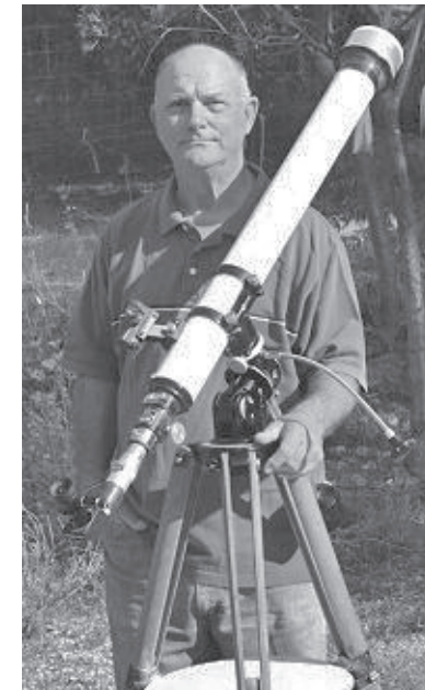
Figure 1: Grisham with his modified 1960's vintage three-inch Tasco telescope on its optional tripod. Normally it is installed on a permanent steel pier imbedded in concrete. Its air-spaced objective provides remarkably sharp images.
